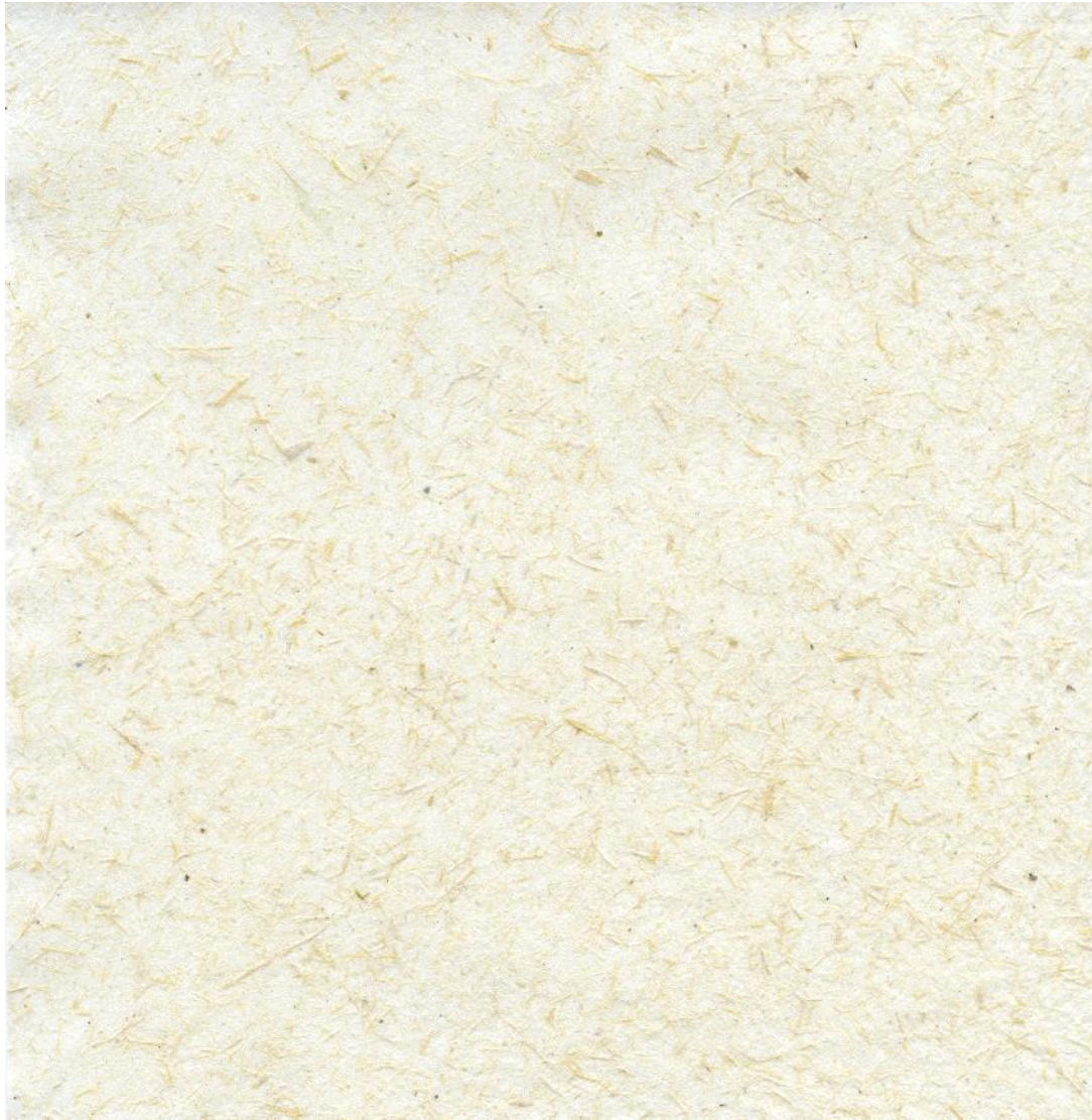
Paper with cucumber stem fibre bundles. Calendered sheet.
