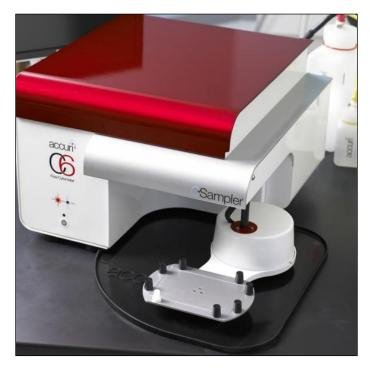
Figure 1-8. BD CSampler with Mat Installed
