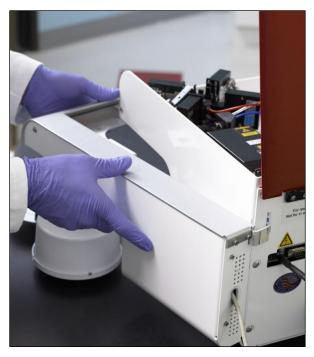
Figure 1-4. Insert BD CSampler Tab into Flow Cytometer
