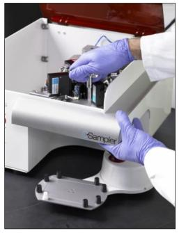
Figure 1-5. Secure the BD CSampler to the Flow Cytometer
