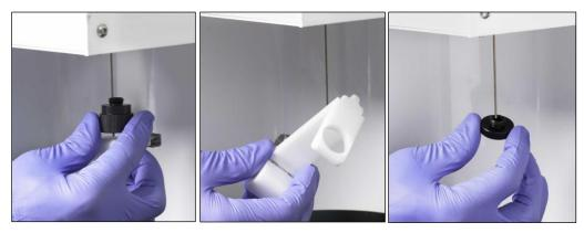
Figure 1-2. Installing the BD CSampler SIP Collar
