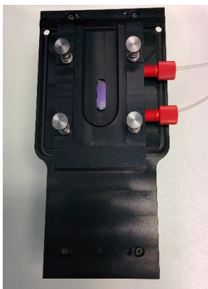
Figure 5.15 O-Ring top-plate with tubing fittings for syringe pump use.
