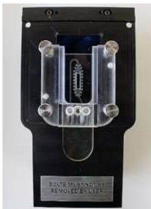
Figure 5.10 Low Volume Flow Cell assembly mounted on laser module with sprung fastening bolts.
